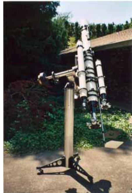
Unitron 5" f/16 refractor telescope tube assembly and auxiliary equipment remounted on a Meade Research Grade Equatorial. A superb performer, this jewel of a refractor is a favorite for double star hunting.
