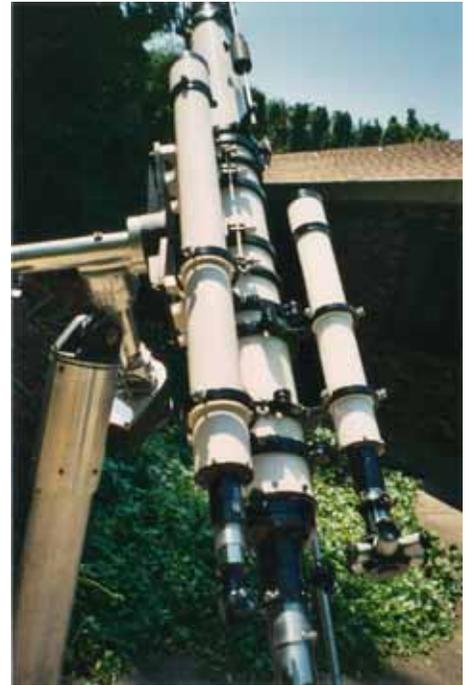
Unitron guide telescopes: 75mm f/16 (left) and 60mm f/11.7 (right).
