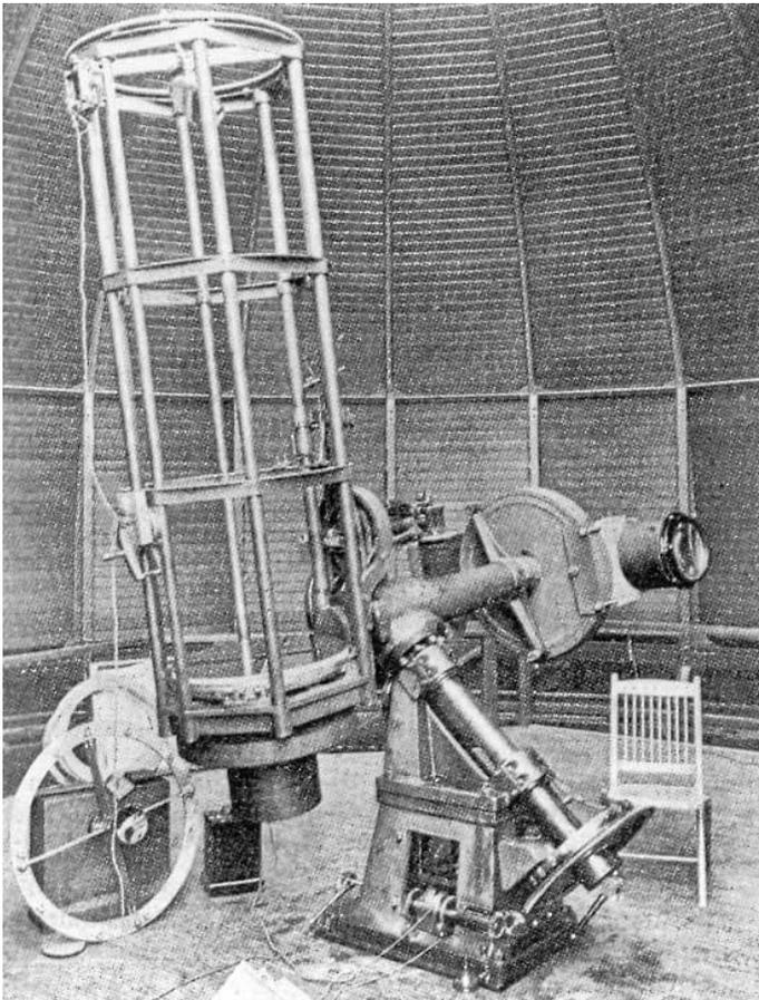
First of all, the utter familiarity of the design is striking. The scope is set up as a Newtonian, but note the Cassegrain secondary cage and mirror at the bottom left of the photo. Right next to it is what looks like a battery for the motor drive. There also seems to be a camera attached to the counterweight. The optical assembly is remarkable in that the six tube open frame work tube is a design that's been making a comeback lately in amateur scopes of similar size.
